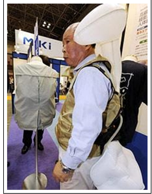
Figure 2. An airbag created for elder by Prop, a Tokyo-based company, which can inflate in 100 ms, if the user starts moving quickly toward the ground. 19
